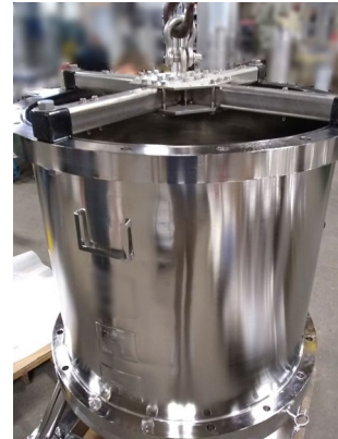
Using the lifting device to place the body on the outlet head
