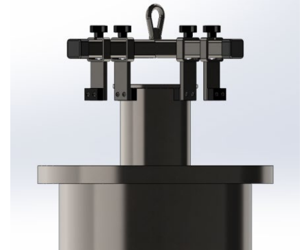
Using the lifting device to remove the inner frit
